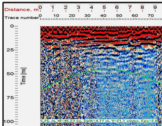
Figure 6: Profile N0.314 after the Apply Background Removal
