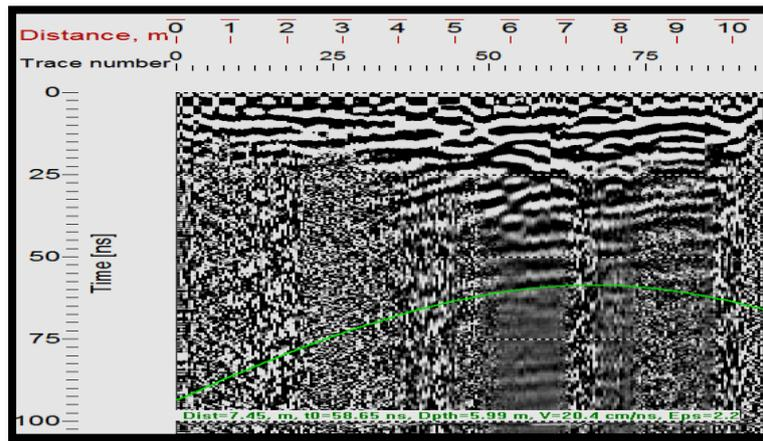
**Figure 7: Profile N0.315 after the Apply Background Removal**
