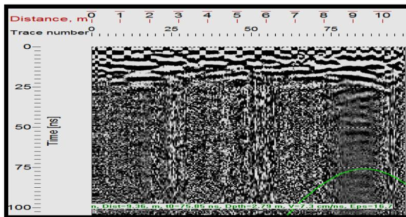
Figure 10: Profile N0.316 after the Apply Background Removal
