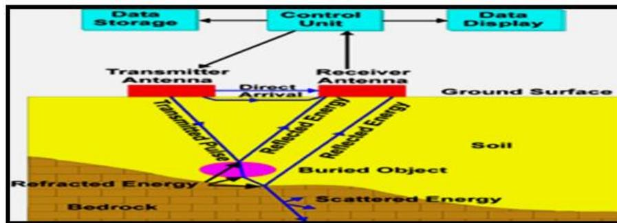
Figure 1: Basic Principle of GARR [6]
