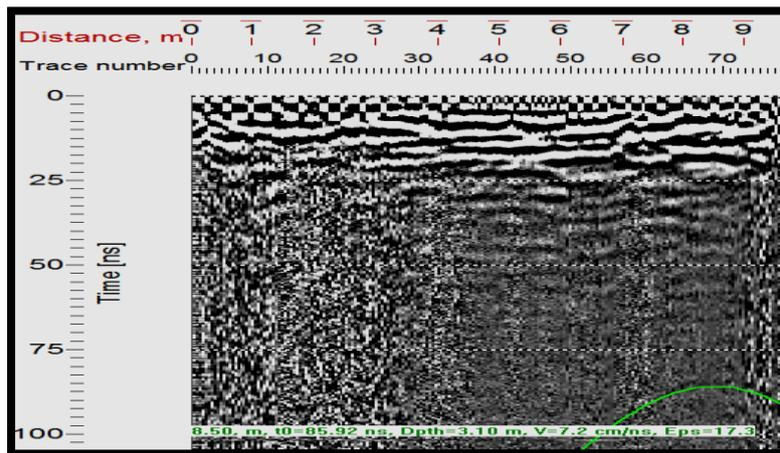
**Figure 8: Profile N0.314 after the Apply Background Removal**
